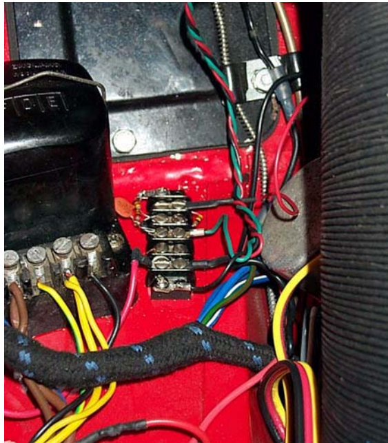
Figure 11. Pulse-cleanup circuit installed in the car. The twisted set of wires goes to the tachometer. Red and black are dc power and green is the triggering pulse.
